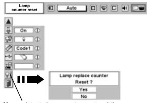
Move pointer to Lamp counter reset and then press SELECT button. Message "Lamp replace counter reset?" is displayed.
